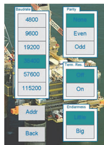
This image is shown when touching the "Modbus" cell in the set up menu screen. Here is possible to set Modbus communication parameters as baudrate, parity, terminal resistance, endianness and address, touching related cells. These parameters are saved in PSO1250 memory and also held after AC1 and AC2 supply shutdown.
