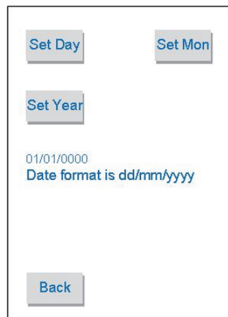
This image is shown when touching the "Set Date" cell in the set up menu screen. Here is possible to set Day, Month and Year touching related cells. Date format is day/month/year (as dd/mm/yyyy). Current setting is shown in numeric format. Date is not kept after AC1 and AC2 supply shutdown.
